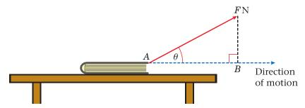
The effect of the force in the direction of motion is the length of the line AB. This is called the **component of the force in the direction of motion**. Using the rule for a right-angled triangle  $\cos \theta = \frac{adjacent}{hypotenuse}$  you can see that the length of AB is  $F \times \cos \theta$ . Finding this value is called **resolving** the force in the direction of motion.
