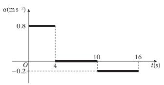
The diagram is an acceleration–time graph to show the motion of a particle. At time t = 0 s, the particle is at rest. Sketch a speed–time graph for the motion of the particle.
