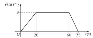
The diagram shows the speed–time graph of the motion of a cyclist riding along a straight road. She accelerates uniformly from rest to  $8 \, \mathrm{m \, s^{-1}}$  in 20 s. She then travels at a constant speed of  $8 \, \mathrm{m \, s^{-1}}$  for  $40 \, \mathrm{s}$ . She then decelerates uniformly to rest in 15 s. Find
