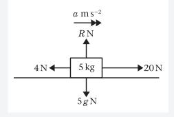
Draw a diagram showing all the forces and the acceleration.
