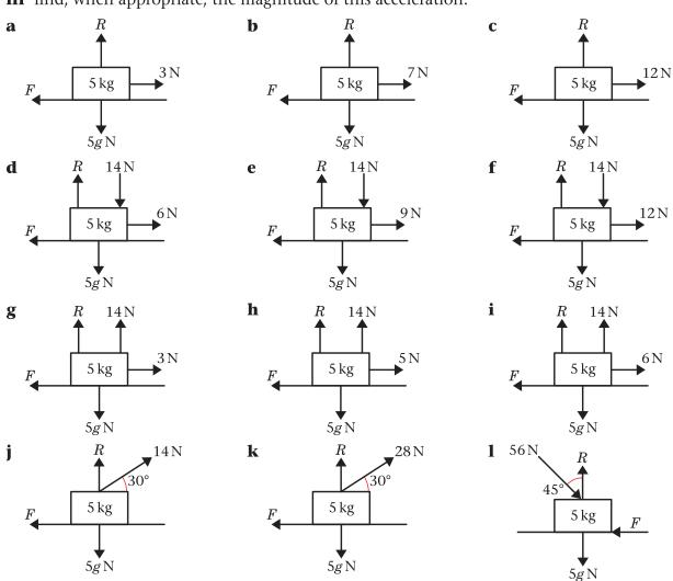
**2** In each of the following diagrams, the forces shown cause the body of mass 10 kg to accelerate as shown along the rough horizontal plane. *R* is the normal reaction and *F* is the friction force. Find the coefficient of friction in each case.
