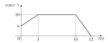
A particle moves  $100 \,\mathrm{m}$  in a straight line. The diagram is a sketch of a speed–time graph of the motion of the particle. The particle starts with speed  $u \,\mathrm{m}\,\mathrm{s}^{-1}$  and accelerates to a speed  $10 \,\mathrm{m}\,\mathrm{s}^{-1}$  in 3 s. The speed of  $10 \,\mathrm{m}\,\mathrm{s}^{-1}$  is maintained for 7 s and then the particle decelerates to rest in a further 2 s. Find
