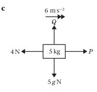
**8** In each of the following situations, the forces acting on the body cause it to accelerate as shown. In each case find the mass of the body, m.
