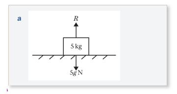
First draw a diagram showing all the forces acting on the block.
